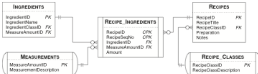
Figure 9–7—The tables you need from the Recipes sample database to fetch all the information about recipes
